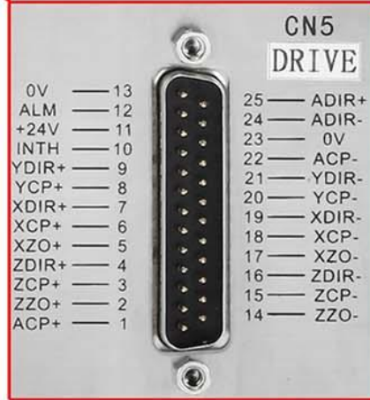
CN5 for control servo/step drivers & servo/step motors.
