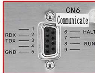
CN6 for connecting to PC & External Switch.
