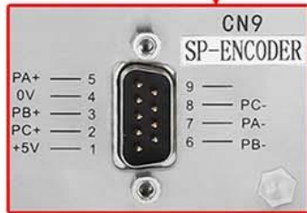
CN9 for connecting to spindle encoder.
