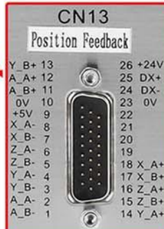
CN13 for connecting to Linear Scale.
