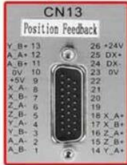
CN13 for connecting to Linear Scale.
