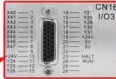
CN16 for connecting to External Switches & Loads
