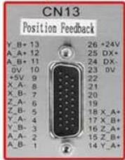
CN13 for connecting to Linear Scale.
