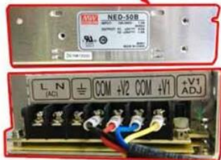
MEANWELL Brand Power Supply (Wide Voltage input:100-240VAC)
